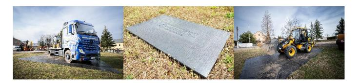
On rugged, unmade terrain, the clickPROtec special load spreading plate ensure a stable base. This is especially important for large machinery, such as cranes, to prevent the support stands from sinking into the ground. The lightweight glass fibre-reinforced material ensures that the panels can be laid manually by one or two employees. They are also easy to transport thanks to their compact dimensions and low base wall thickness of just 15 mm.
